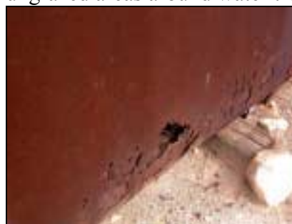
holes rusted through tank
