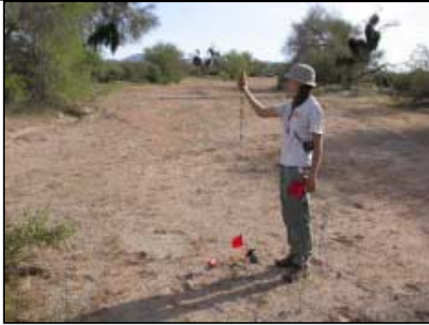
Locating and recording the center of a natural community condition assessment plot using a Garmin eTrex GPS receiver.
